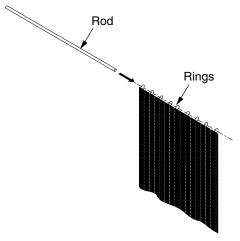
Figure 12 - Assembling Rod and Screen
